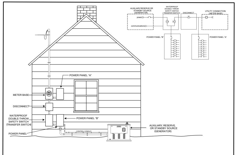
Notes: For metering, grounding, etc. details see drawings GS1.0 and GS2.0.
